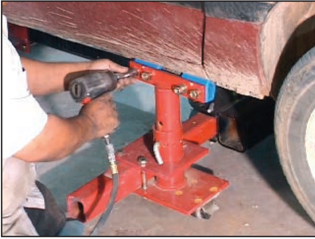
Tighten Pinchweld Clamps securely onto vehicle pinchwelds.
