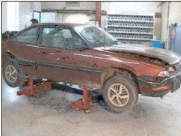
Vehicle is now attached to Spider and you are ready to attach Pulling Towers. Insert tower into desired tower insert and lock into place with locking pin.
