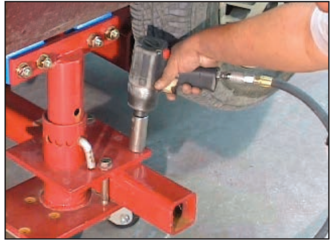
Tighten Pinchweld Brackets securely to Bracket Arms.
