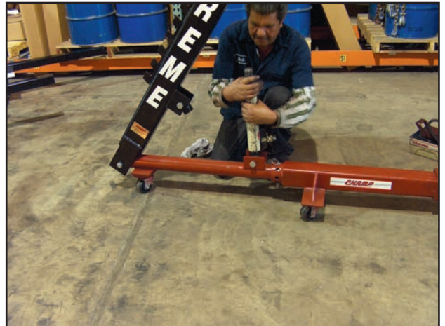
Install Hydraulic Ram by screwing female end to Ram Coupler on Tower Base.
