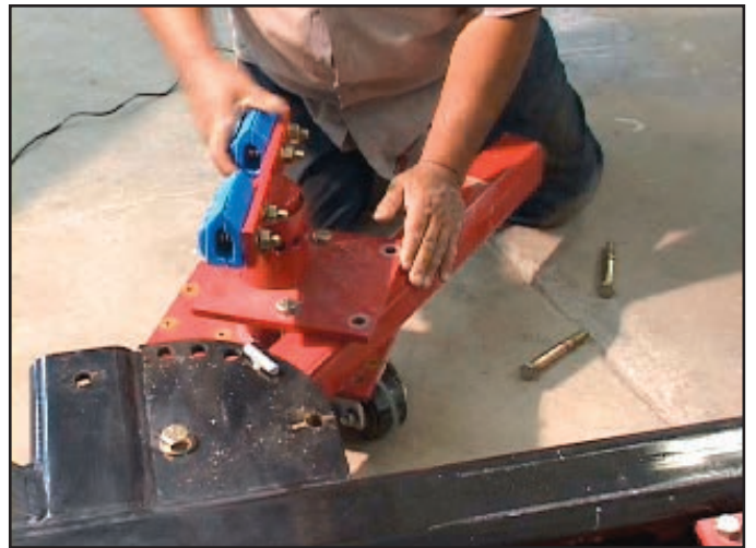
Remove Pinchweld Clamp Brackets.
