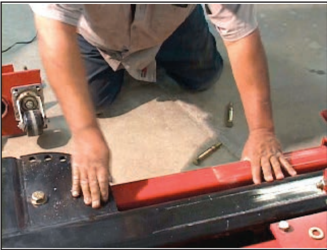
Fold Bracket Arms against Body and lock into place with Locking Pin
