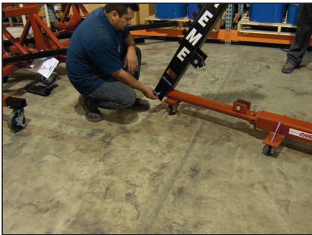
Attach Pulling Tower to Tower Base with supplied bolt. Tighten securely.
