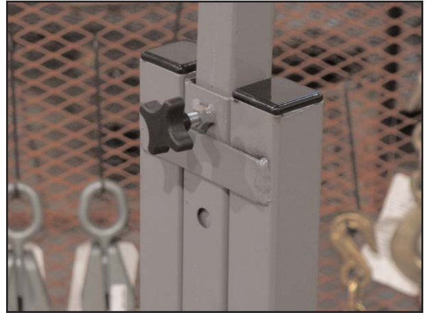
Select desired height of Top Support Extension (C). Insert Knob (F) into top hole of Panel Jack (B), tighten knob to lock Top Support Extension (C) in place.
