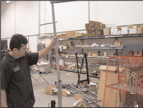
Insert the Top Support Extension (C) into Panel Jack (B).
