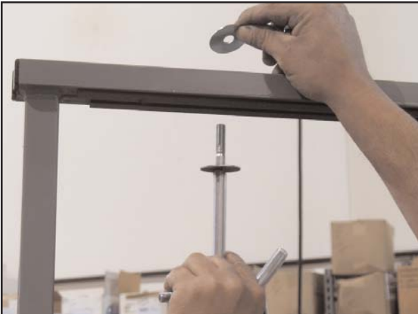
Insert Straight Bolt (G) in between the 2 posts of Top Support Extension (C) and tighten with washer and nut. Repeat for Curved Bolt Assembly (H). Note: Make sure Curved Bolt is in front of Straight Bolt.
