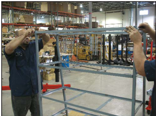
Align Top Support (G) with second set of holes on 28" Upright (B) and bolt into place. Note: Do not fully tighten the bolts.
