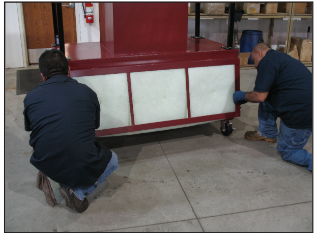
Close hinged panel filter door. Make sure the tri-fold panel filter fits snugly up at the top.
