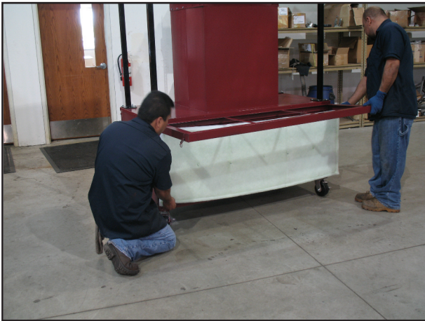
Lay tri-fold panel filter across the front of the carbon filters.
